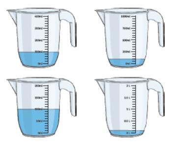
Each of these containers contain the same volume of 100 millilitres but have different capacities and scales. Always look carefully at how the numbers on the scales increase when reading a measurement.
